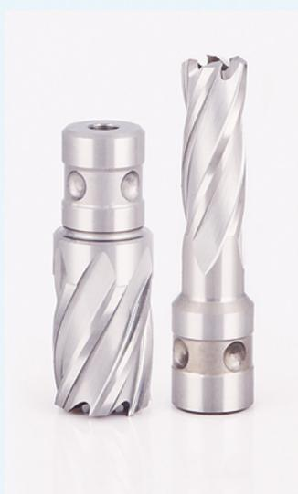
四孔柄系列 柄径 $\Phi$ 18.0mm, 特征在于90度分布4点定位孔。适合用于FEIN系列磁座钻机。HSS annular cutter with FEIN Quick-in Shank, the diameter of shank is  $\Phi$ 18.0mm, which is suitable for 90° distribution at 4 locating holes. FEIN Quick-in Shank, suitable for FEIN magnetic drills.
